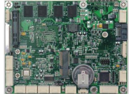
Altair supports 1GB or 2GB of DDR2 DRAM soldered on-board and provides high-resolution LVDS and VGA graphics interfaces. Additional I/O ports include SATA, USB, serial, digital I/O, and dual Gigabit Ethernet. Flexible system expansion is based on stackable EMX modules, and a PCIe MiniCard socket. A socket is also provided for an optional on-board USB flashdisk of up to 8GB.
