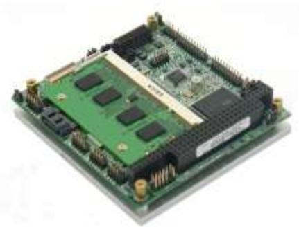
**Diamond's Aurora SBC with RSODIMM memory module installed**
