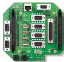
Helios panel I/O board
