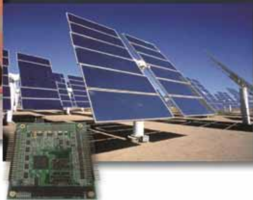
GPIO-MM digital I/O module with custom programmed FPGA provides motion control to aim solar mirror arrays
