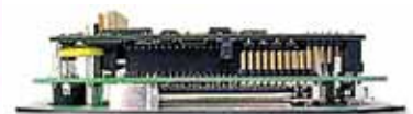
Unique panel I/O board mounting method eliminates cables and mounts the entire system directly to the enclosure front panel
