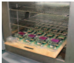
Environmental Test Chamber used for temperature validation, screening, and burn-in activities.
