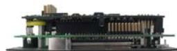
Unique panel board mounting method eliminates cables and mounts the entire system directly to the enclosure front panel
