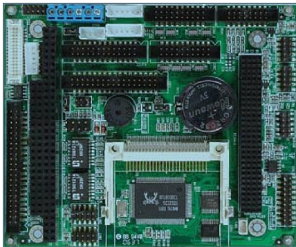
ETX form-factor development kit: Matches the footprint of the ETX-945 and provides connectors for system I/O, CompactFlash, PC/104-Plus expansion, two additional serial ports, RS-232/422/485 buffering, a digital I/O port, and a second Ethernet LAN interface.
