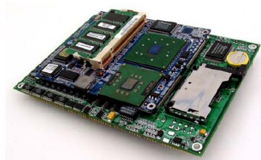
EPIC form-factor development kit: Provides connectors for system I/O, CompactFlash, PC/104-Plus expansion, four additional serial ports, RS-232/422/485 buffering, a second Ethernet port, a 5V/7-28V DC-to-DC power supply, and an industry-leading data acquisition subsystem.
