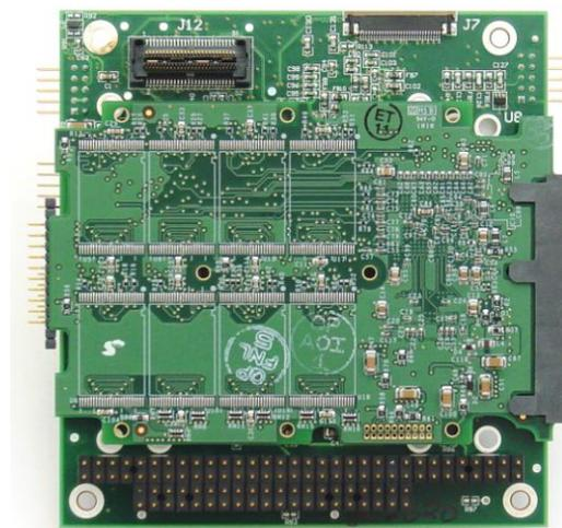
VGA accessory board with SATA SSD installed on the bottom
