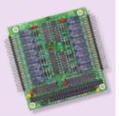
**Pearl-MM** offers 16 SPDT relays with normally closed, normally open, and common contacts for maximum flexibility. All relays are in the normally closed position on power-off and power-up. High reliability components and wide temperature operation make Pearl-MM a rugged solution for your application.
