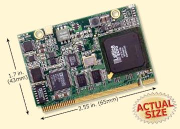
The **FeaturePak** standard, originated by Diamond Systems, provides a compact, low-cost method of adding I/O to board-level embedded computers. The modules can be used as snap-in customization modules for commercial, off-the-shelf single-board computers (SBCs) and computer-on-module (COM) baseboards, or as functional blocks on fully-custom embedded electronics.
