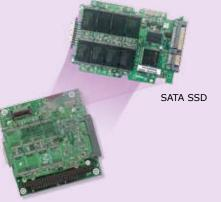
Corona SUMIT Communications module with SATA SSD installed on the bottom.
