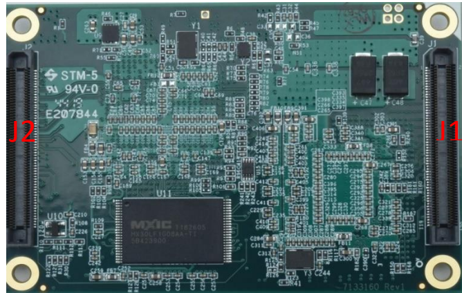
Figure 8-1: EPSM-10GX4 Module B2B Connectors
