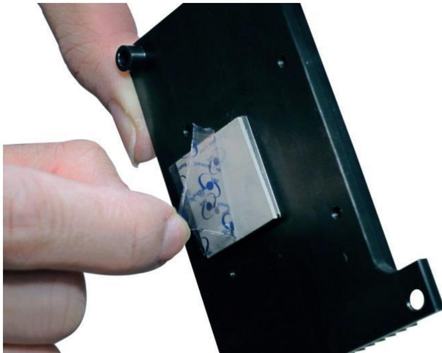
Figure 22 Remove plastic foil from the TIM
