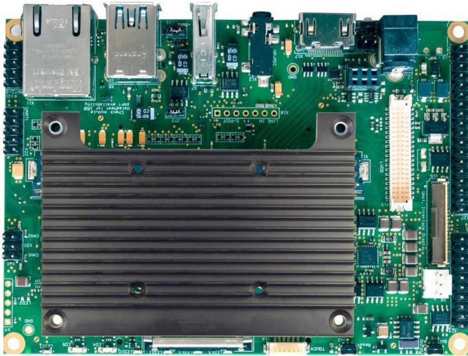
Figure 23 Align heatsink screw holes with the fasteners
