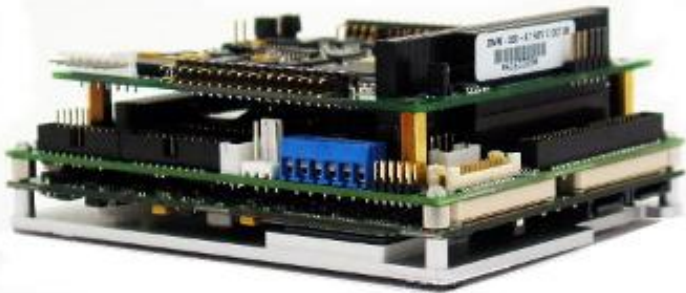
Standard Embedded-Ready Subsystem + PC/104 expansion module
