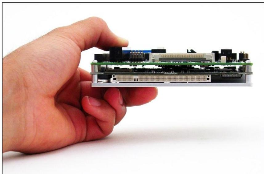
**Figure 1: Edge View of the Pluto Embedded Platform**
