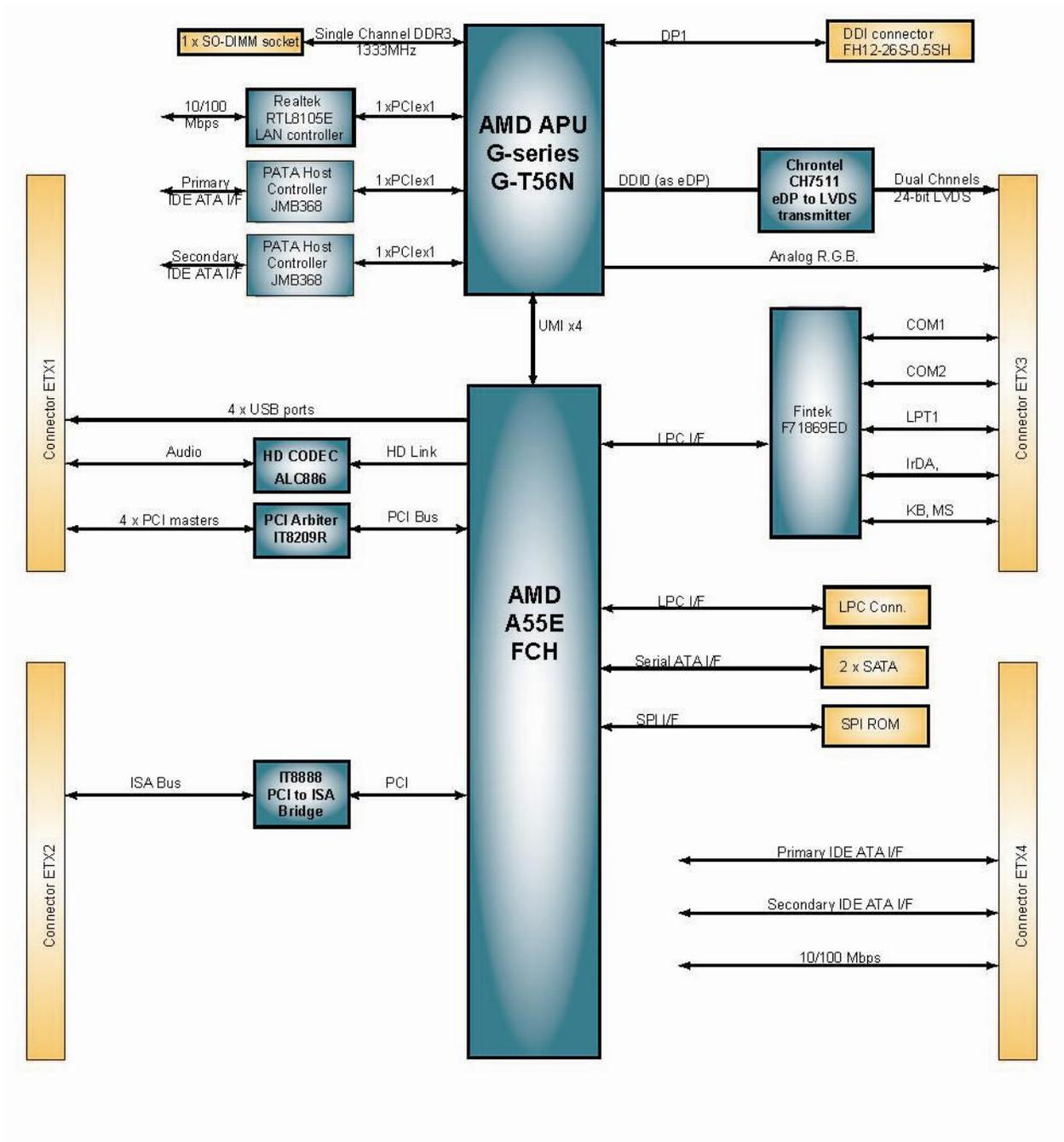
**Figure 3: Typical ETX CPU Module Functional Block Diagram**
