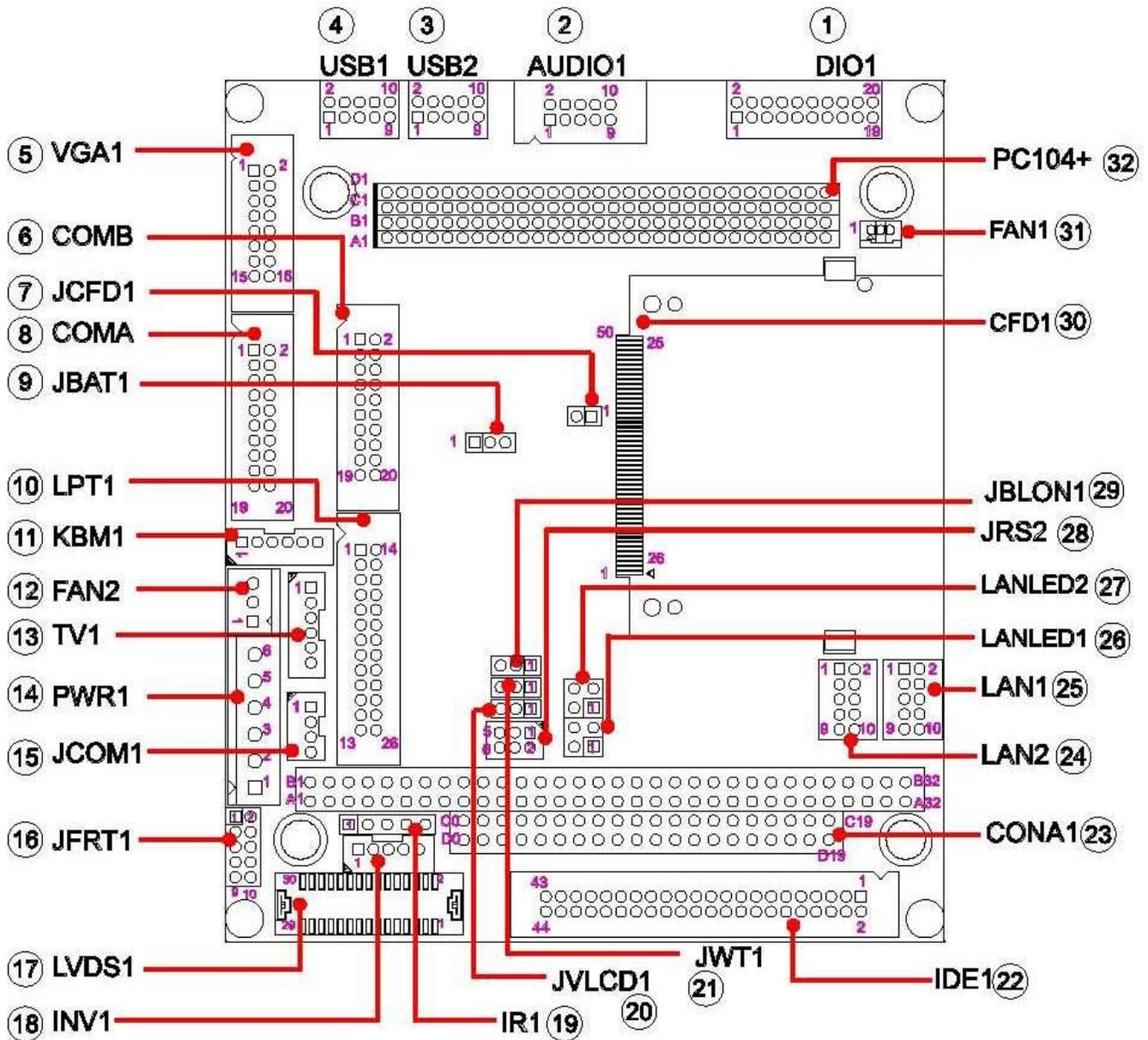
**Figure 5: Baseboard Connectors and Jumpers**
