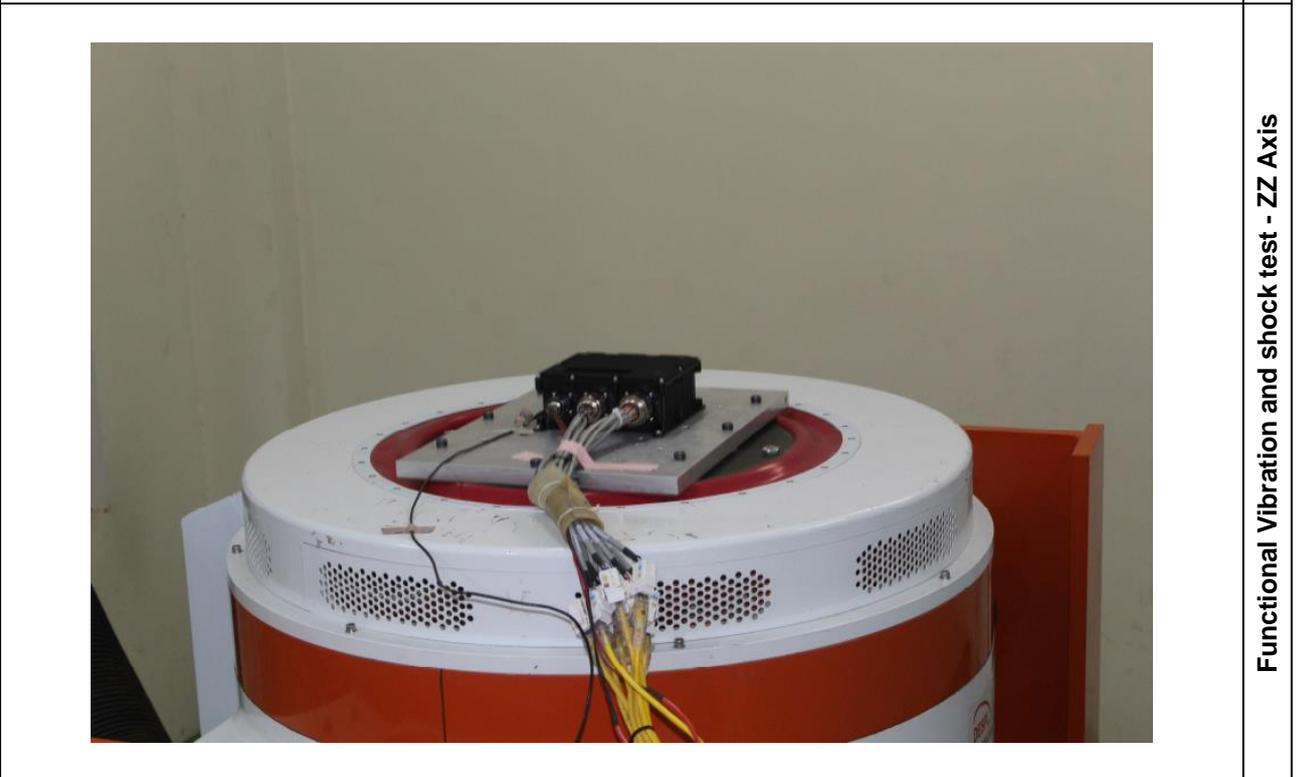
Functional Vibration and shock test - ZZ Axis
