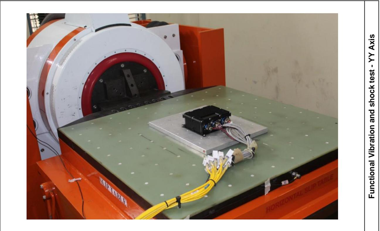
Functional Vibration and shock test - YY Axis
